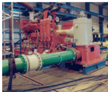
SPP Vertical Turbine pump on test
