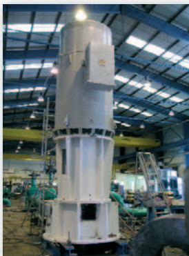
SPP vertical lineshaft pump directly driven by a 1200kw electric motor
