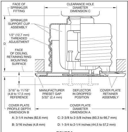
FIGURE 2 SERIES RFII-MRI CONCEALED SPRINKLER INSTALLATION DIMENSIONS
