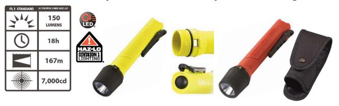
Material/Lens Impact and chemical resistant Engineering Polymer resin; o-ring sealed and vented. Available in high visibility yellow or orange. Unbreakable polycarbonate lens with scratch resistant coating
