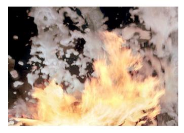
Great extinguishing power even on light hydrocarbons and gasoline containing additives such as TBA or MTBE that, due to their foam destroying action, make the extinction particularly difficult when using conventional synthetic or standard protein foam concentrates.
