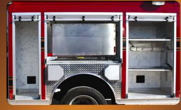
Loads of storage - swing out tool board, two (2) adjustable shelves and SCBA tubes located in wheel well.
