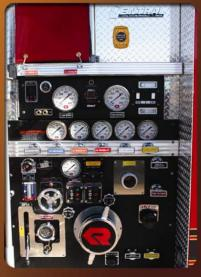
PTO & Midship pumps up to 1000 GPM. Foam and generator systems (120/240 volt) also available.
