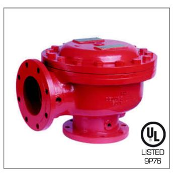
Deluge Valve is known as a system control valve in a deluge system, used for fast application of water in a spray system. Deluge valve protects areas such as power transformer installation, storage tank, conveyor protection and other industrial application etc. With the addition of foaming agent they do protect aircraft hanger and inflammable liquid fire.
