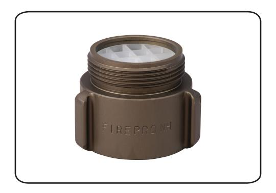
Mini Stream Shaper lightweight aluminum or brass body with hard anodized finish and replaceable Delrin "Honeycomb" grid straightens stream minimizing water turbulence, resulting in improved, effective distance and overall reach.
