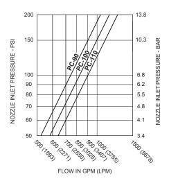
WATER OR FOAM SOLUTION NOZZLE DISCHARGE CHARACTERISTICS
