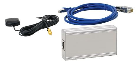
The time control module is connected directly to the DOM4- 8/4-24 and ensures time synchronization via GPS signal. This facilitates exact timing of automated announcements (e.g. school bells), timed volume a justments (e.g. reduction of volume level at night for train stations) or simply the exact documentation of announcements or malfunctions.
