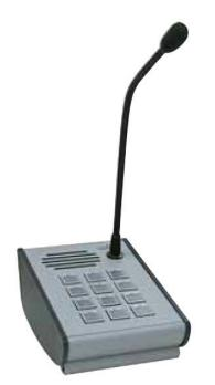
The paging microphones DCS15 and DCS2 with the paging microphone keyboard module DKM18 allow for the selection of loudspeaker circuit, the transmission of voice announcements as well as various gongs and alarms. Each microphone is connected to the available DAL-bus (Digital Audio Link) on the DOM (Digital Output Module) via a standard Cat5 cable. All control signals as well all audio signals are transmitted digitally.
