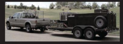
The Falcon FSD5" is a large-scale Compressed Air Foam (CAF) truck and trailer system capable of dispersing standard fire suppression foams, Hazmat foams and biological and chemical warfare decontamination formulas.
