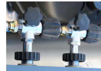
Safety filling connection
