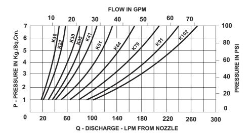
$Q = K\sqrt{P}$  where P is supply pressure in Kg/sq.cm., K= nozzle constant (K-factor) in metric US K factor = Metric K factor  $\div$ 14.2745
