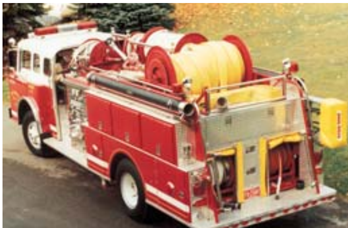
Pumper with six reel units—1" booster hose to 4"LD collapsible hose.
