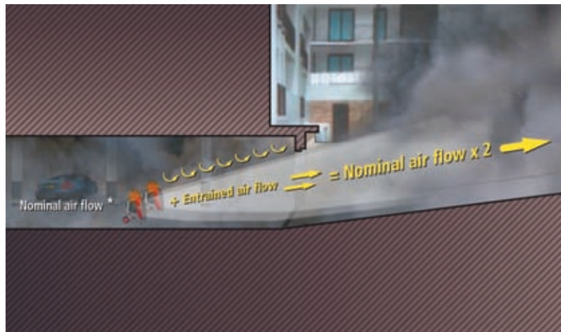
Fig 1 : 2 CarPark Fans in action
