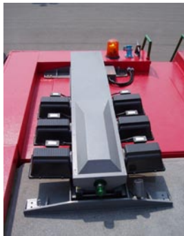
Detailed view - front nozzles of the self-protection system
