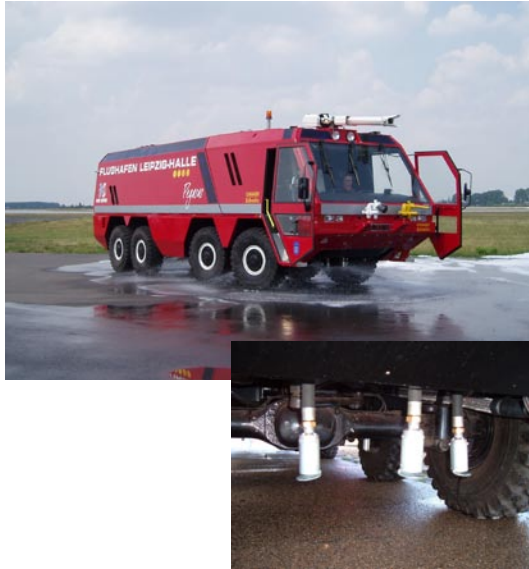
Detailed view - front nozzles of the self-protection system
