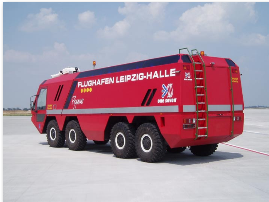
The air-crash tender of the airport Leipzig - Halle FLF 80/125 One Seven® „PEGASUS“
