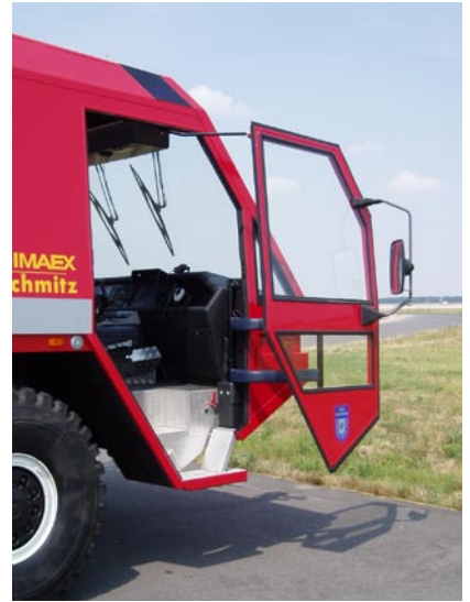
Detailed view of the pneumatically opened driver's door
