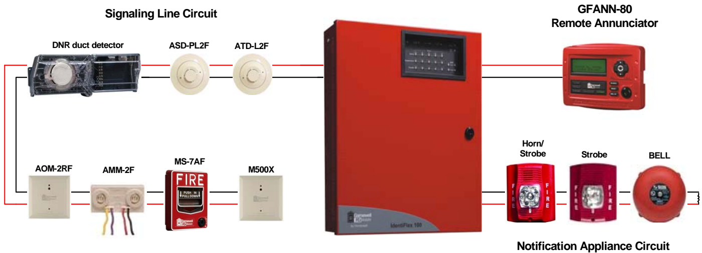
Figure 1 IdentiFlex 100 Addressable FACP Overview
