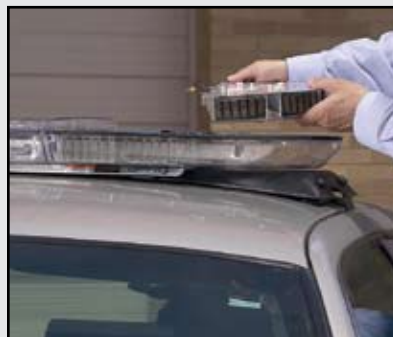
2 Disconnect the ROC board by the 22-gauge wire harness.
