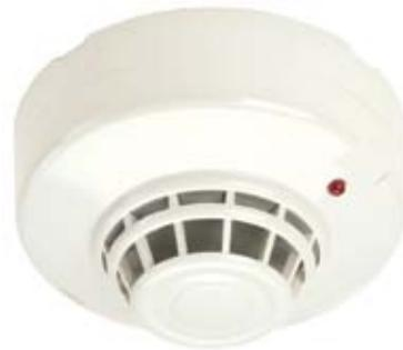
The Edwards SC20FTU-3 is a fixed temperature heat detector, with an alarm threshold, operating at 135°F (58°C).
