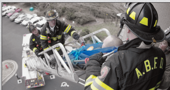
Fly section wide enough for a stokes basket between the handrails.
