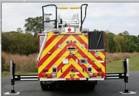
Pin-free jack system deploys in under 40 seconds
