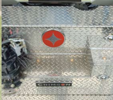
Removing (4) screws gives you total access to drive gears for simple adjustments.
