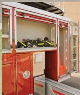
Maximum storage, the X-Style Outrigger System leaves room for full height, length and depth storage.
