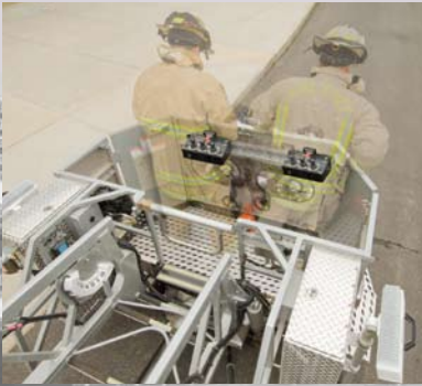
Sliding aerial controls provide optimum platform operating view.
