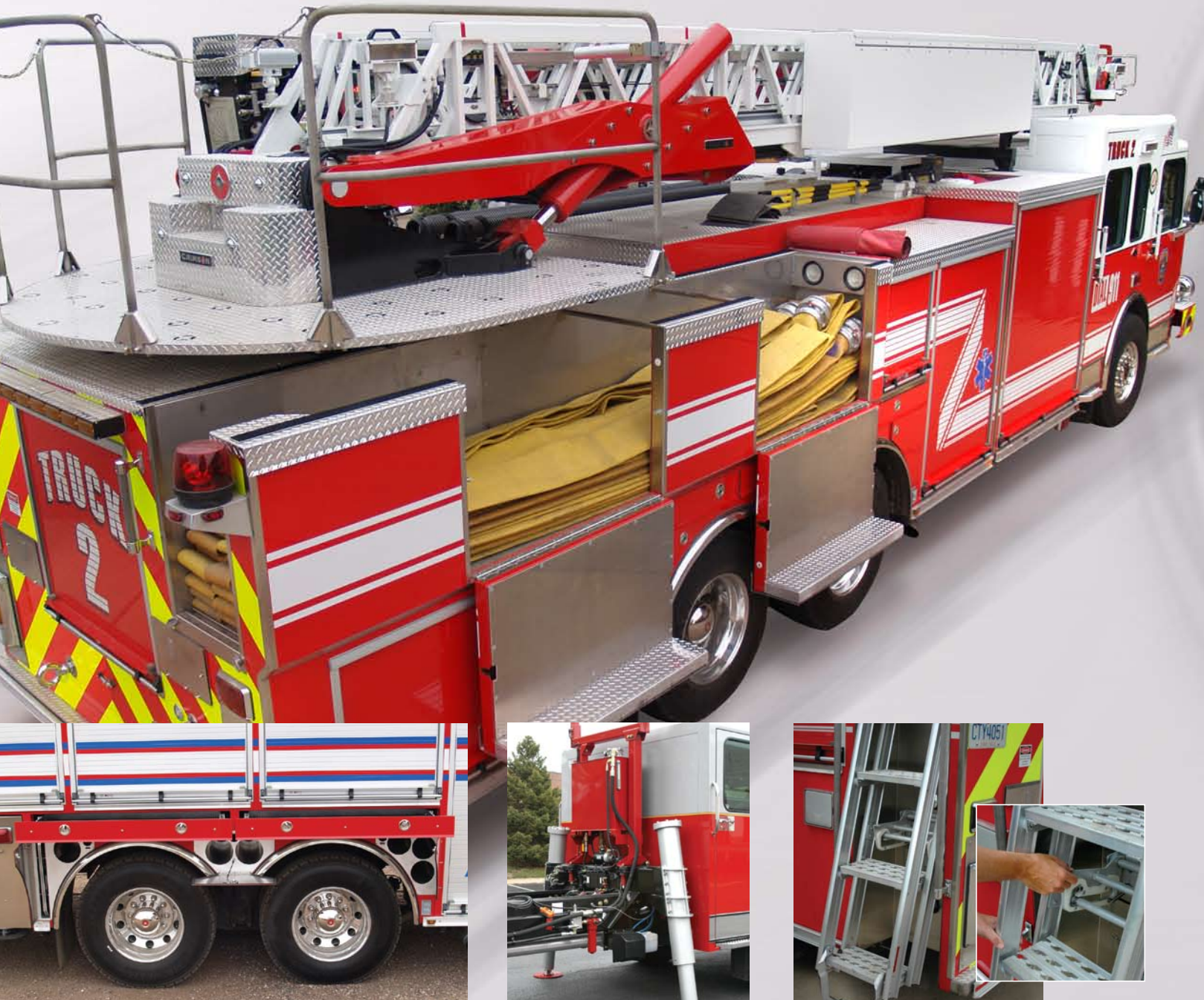
Storage around the wheel wells increases the amount of usable storage space.
