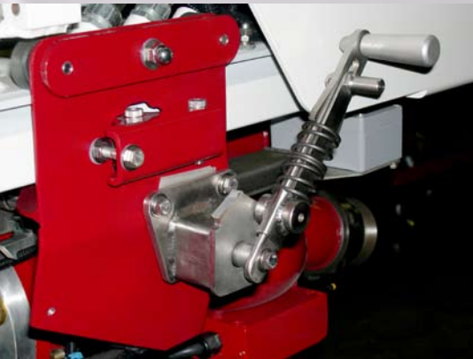
Locking waterway nozzle mechanism
