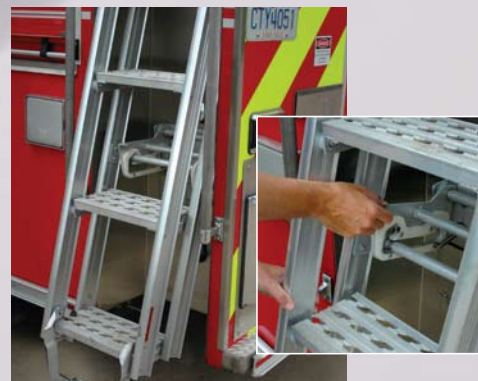
Ergonomically designed easy pull out Turn Table Access Steps increase safety.
