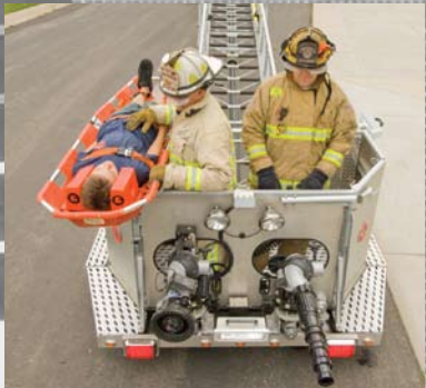
Stokes Basket brackets and sliding aerial control provide the ultimate rescue platform.
