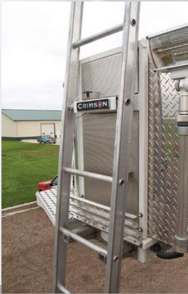
Parapet Rescue brackets provide convenient roof ladder mounting
