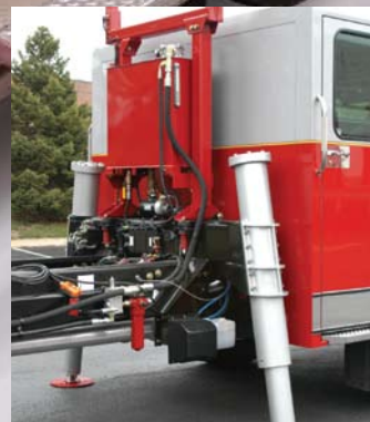
Ladder Travel and Rest Cradle incorporates Crimson's Vibra-Torq™ to eliminate ladder and cradle stress.
