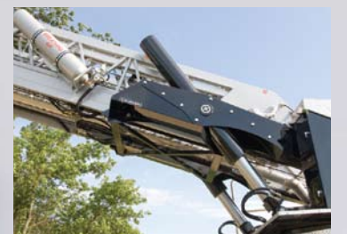
Patented Lift Cradle positions the ladder close to the ground, making it possible to safely add or exchange equipment at the tip of the ladder. It also enables the ladder to lower to negative 10 degrees for low-angle operating conditions.
