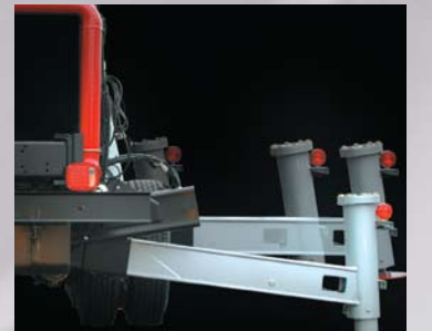
Crimson's innovative outriggers allow the apparatus to level on slopes up to 15 degrees and handle truck set-ups on severe terrain. This X-Style Outrigger Leveling System will allow you to safely set up your aerial in situations you've never before thought possible.
