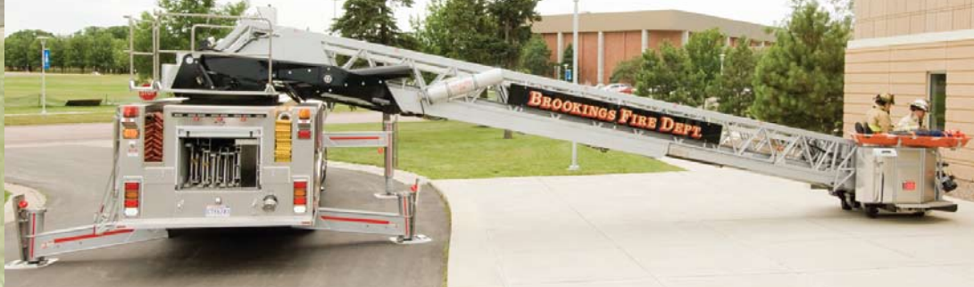
The Crimson Platform can rest on the ground while fully retracted, allowing you to squeeze into tighter spaces in the field.
