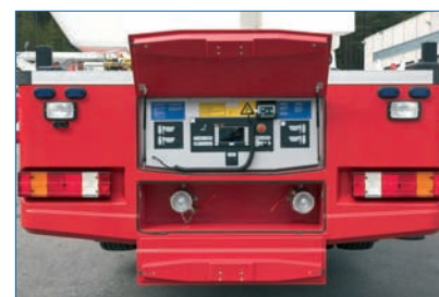
Single operator outrigger controls. Option for integrated water inlets.
