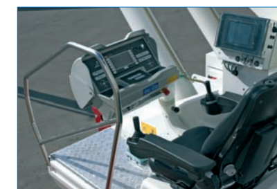
Option for integrated control levers at armrests.
