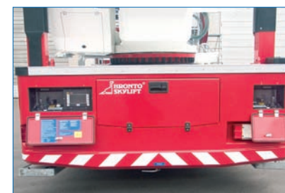
Well protected outrigger controls on the both sides also available.
