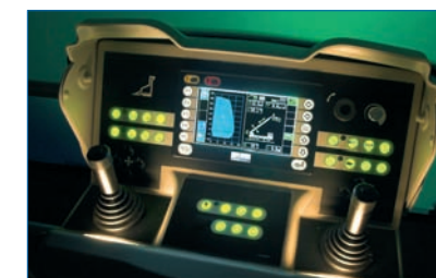
All RLX units have Bronto+ electronic control system. Control centers have full colour displays with excellent visibility.
