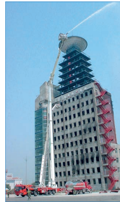
HLA units are purpose-designed for rescue and fire fighting with integrated waterway.
