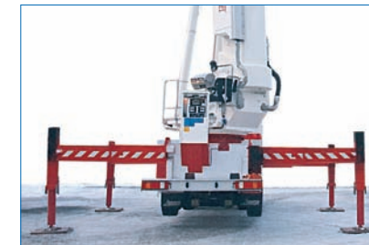
With the easy automatic levelling function the unit is fully stabilized for rescue in 40 seconds.
