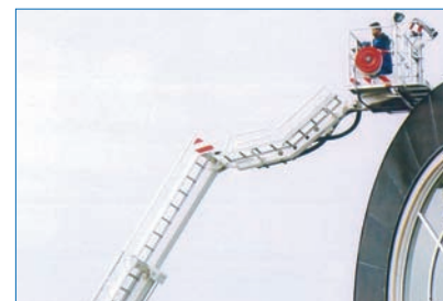
Integrated rescue ladder according to the latest European Norm.
