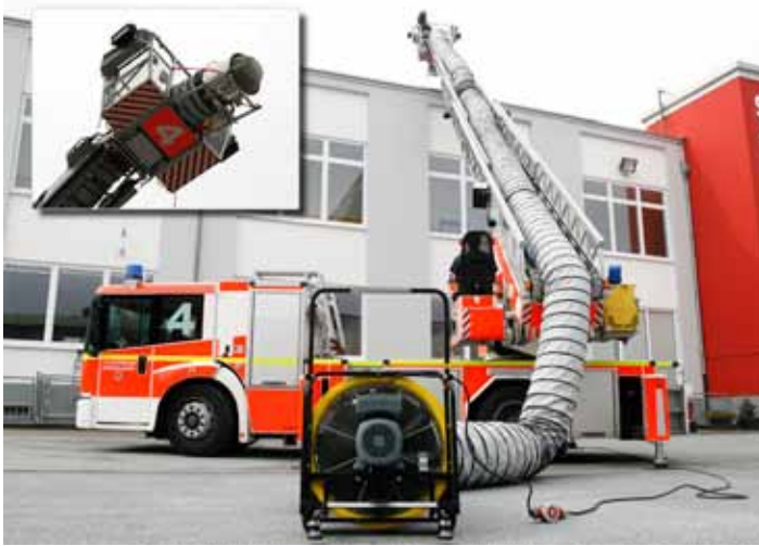
Use of the foam generator system on a aerial ladder
